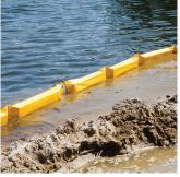
**TURBIDITY CURTAINS** A flexible, impermeable barrier that is weighted at the bottom. Contains sediment and silt stirred up by construction activities in or near bodies of water, dredging operations and rainwater runoff.
